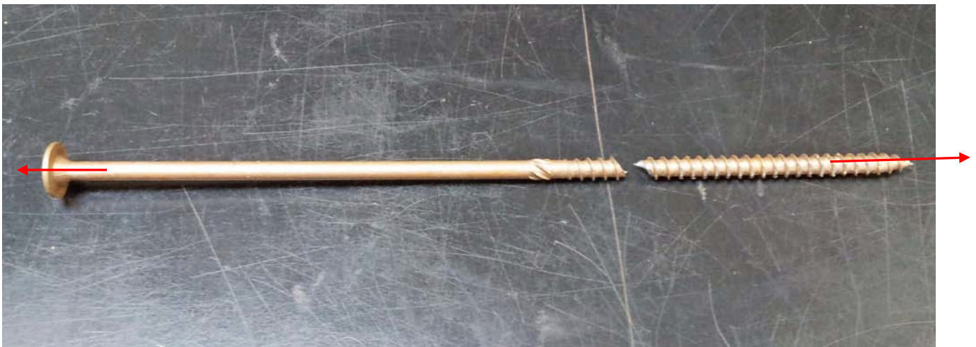
Figure 2 – A setup photograph for tensile testing, in accordance with AISI S904-08. A CTX 381000 specimen is shown. The red arrows show the direction the force was applied.
