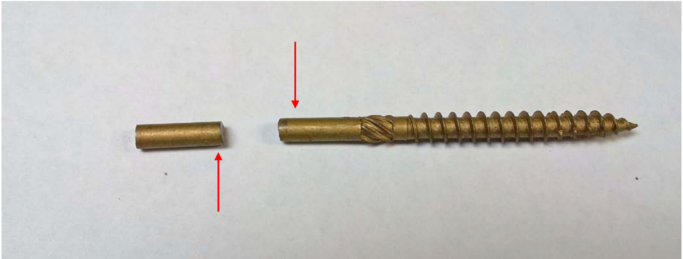
Figure 3 – A setup photograph for shear testing, in accordance with AISI S904-08. A CTX516400 specimen is shown. The red arrows show the direction the force was applied. The head was cut off of the specimen to allow for ease of loading into the fixtures.
