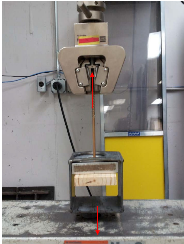
Figure 5 – A setup photograph for head pull through testing, in accordance with ASTM D1037-12. A CTX 381000 specimen is shown. The red arrows show the direction the force was applied.
