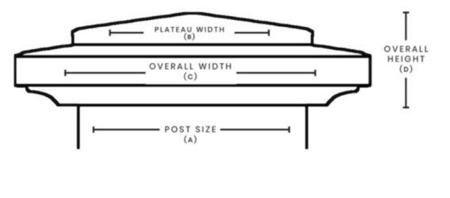
MEASUREMENT DIRECTIONS Measure the **actual width** of your post and order according to the **post size** chart.
