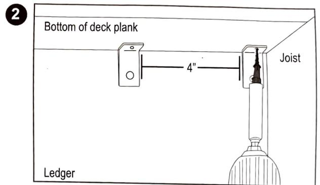
Then use the 3/4" plank screw to attach the L-Bracket to the underside of the plank.
