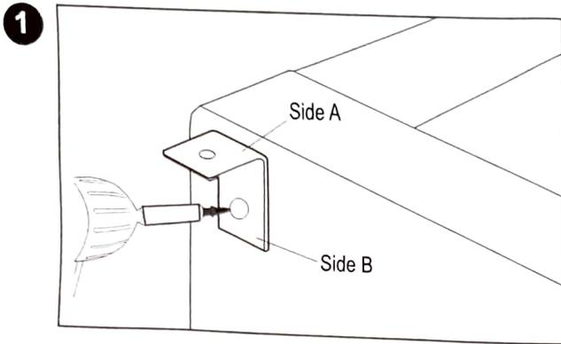
Use the 1-1/2" joist screw provided to install the L-Bracket into the outside of the rim joist.
