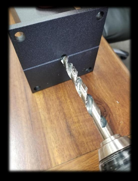
Prepare any post that will receive lighting by drilling the bottom hole to ½"
