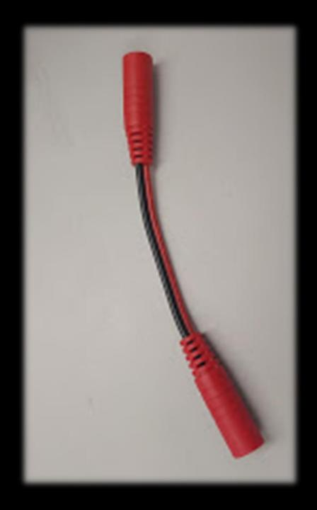
Pictured is a closed loop connector. It is an optional accessory that is included with the SMARTPOWER 50 transformer. It fixes voltage drop issues when a run is too long, or houses too many lights for one main harness to handle.
