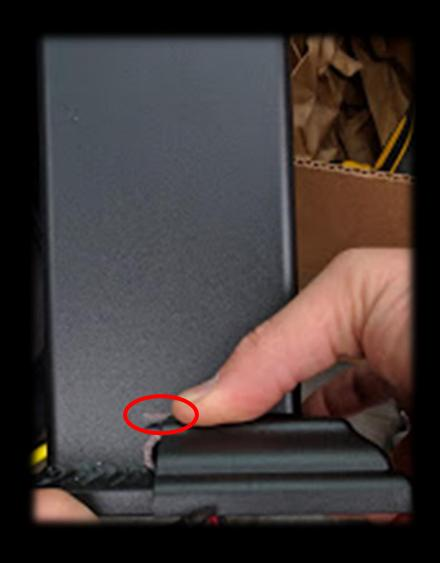
Mark where the top the of skirt is on the post to ensure the hole for the harness is not visible after the installation.
