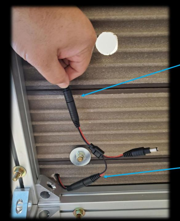
Connect the male end from the main harness to the female connector on the 2 output splitter.
