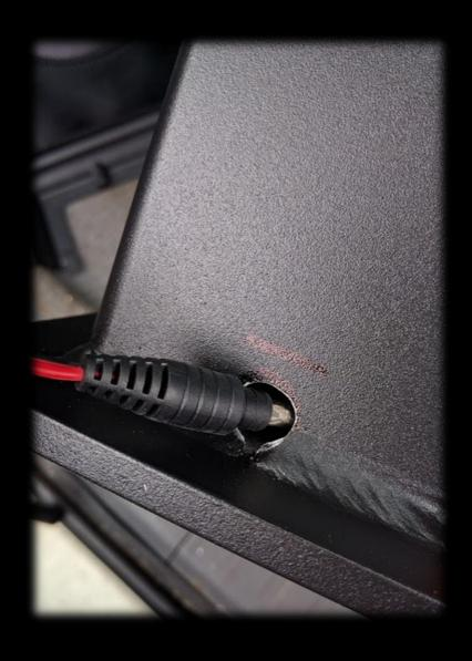
Insert the harness into the drilled hole at the bottom of the post.
