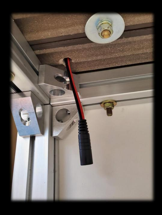
PHOTO: Female connector and harness, below deck surface.
