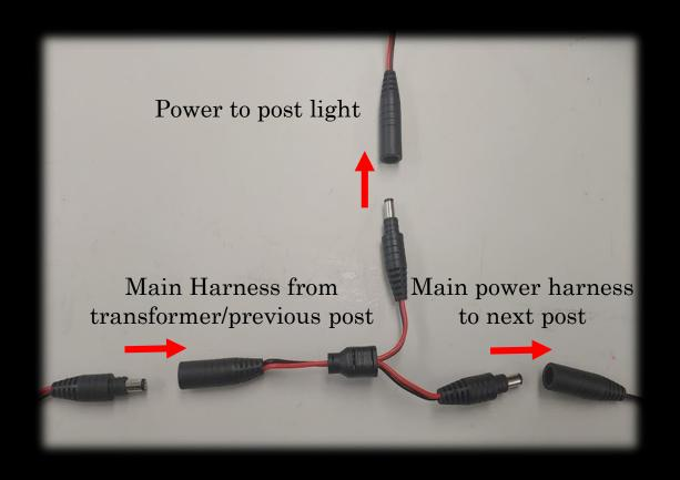
Use a 2 Output Splitter to continue the harness to the next light, and to connect the light placed on the post to the existing harness.
