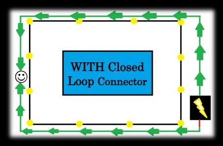
EXAMPLE: The closed loop connector takes a run of 12 lights around a pool, and breaks it into 2 separate runs of 6 lights each, lightening the load on the single main harness. It essentially acts as an additional 'main harness' in the lighting system.
