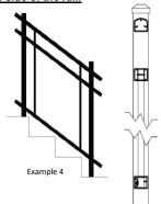
Position rails against posts and even the end spacing on each end, *if possible*, with balusters parallel to the post. Clamp rails to post (Example 4). Mark rails for cutting (Example 5). Mark posts for each mount position (Example 6). Cut rails 3/16" shorter than mark on each end. Rails should be cut using a straight cut.
