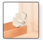
Slide the Aluminum Base Channel behind the Plinth Base tabs.
