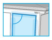
• Once the Vinyl Cap is secured at the corners move to the center and again secure screen by pressing or tapping the Vinyl Cap with a rubber hammer. Next tap from the center out towards each corner. Double check that Vinyl Cap is secure and the screen fabric is still square
