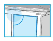
• Square the included screen fabric to the TOP of the panel and attach to the Aluminum Base by pressing or tapping the Vinyl Cap with your hand or rubber hammer to the corners first for about 3"
