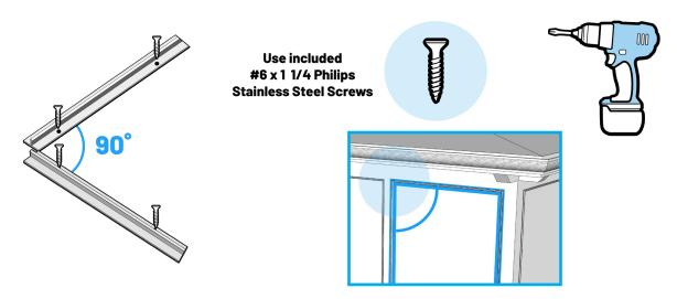
• Secure the Aluminum Base to the porch post with included screws - Pre-drill pilot holes to prevent edge splits at your screw centers
