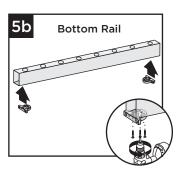
**NOTE:** For ease of bracket attachment place rail against stationary flat vertical surface along with bracket.
