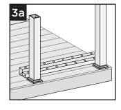
3b.Also allow for a minimum of 1-9/16" (40 mm) on each end of rail for bracket placement AND baluster clearance. Mark rails at intersection of rail and post.
