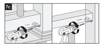
7c.Install both bottom and top brackets on each side to post using two #8-10 x 2" wood screws (provided).
