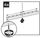
4b. Keeping bottom rail inverted, Use same drill bit, center and drill weep holes through bottom rail at 4 evenly spanned locations to allow for water drainage.
