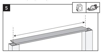
5. Cut deck boards to appropriate length of railing span, remembering to include extra space on each side of the deck board to allow for attachment to the post. Decking boards must cover 1/2 of the pressure-treated post to allow this to be fastened later.
