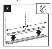
8. Secure deck board to Select top rail with 3/4" screws provided approx. every 16" on center. Screws are to be installed inside of the baluster holes into the decking board. **DO NOT** overtighten.
