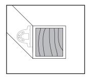
place. Before attaching bracket to rail, measure and mark to ensure bottom rail remains parallel to upper rail.
