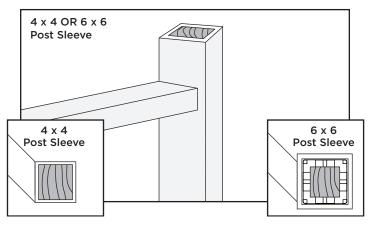
Both 4" x 4" (102 mm x 102 mm) or 6" x 6" (152 mm x 152 mm) post sleeves work well for angles up to 45 degrees. Bottom rail brackets may need to be slightly offset to one side in order to fit properly to hold rail in
