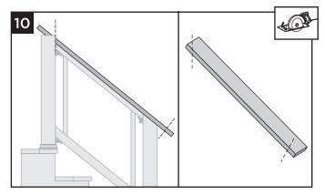
10.Measure accordingly and cut deck boards to appropriate length of railing span also allowing for additional decking material that will be installed over the lower stair rail post.
