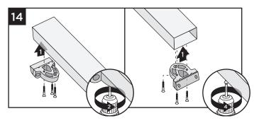
14. On the TOP RAIL, attach the assembled stair brackets to the side WITH the baluster holes. Attach both brackets using three #8-18x1" self-drilling screws (provided).
