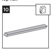
Place inverted Select top rail (orient properly so baluster holes are shown top side up) on 2 x 4.
