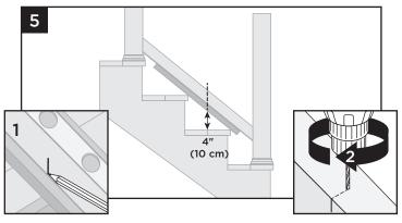
5. Mark approximate location for foot block, allowing a measurement of 4" maximum. Invert the bottom rail. and at marked location drill a hole using a 3/16" drill bit in the center of the channel. Foot block is to be installed at last step.
