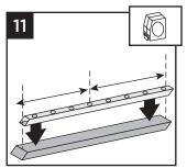
12. Secure 2 x 4 to Select top rail with 3/4" screw provided approximately every 16" on center. Screws are to be installed inside of the baluster holes into the 2 x 4.
