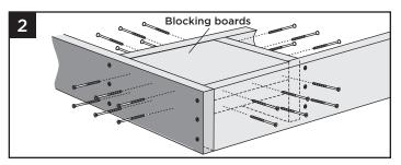
2. Install two 2" x 8" (5.1 cm x 20.3 cm) boards as blocking under post location. Securely attach blocking using a total of twenty-four 3" (7.6 cm) pressure-treated compatible screws (*not provided*).
