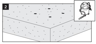
2. Clean out holes to remove all concrete dust.
