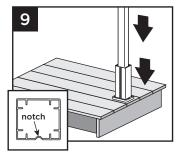
Attach bottom guide block using one 10 x 1" selftapping screw (provided) in notch to lock guide block onto post.
