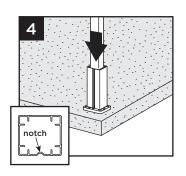
Attach bottom guide block using one 10 x 1" (25 mm) self-tapping screw (provided) in notch to lock guide block onto post.
