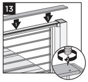
14. Secure boards to top rail using Trex Signature Cocktail Bracket (sold separately). Ensure that there is a bracket at each end of the railing section, then space brackets approximately every 24" and attach with 4 screws provided.
