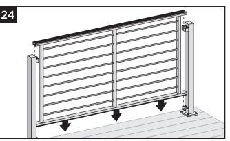
24. Drop assembled rod rail panel into brackets.
