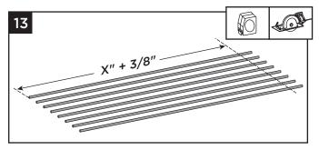
13. Cut rods to the length measured in previous step.
