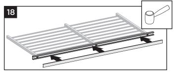
18. Align cover on one side of bottom rail in slot on side of rail. Then starting from one end of rail snap cover onto opposing slot working down the length of rail. In some cases, GENTLE tapping with a rubber mallet may facilitate fastening.
