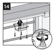
NOTE: Pre-drilling before attachment is recommended.
