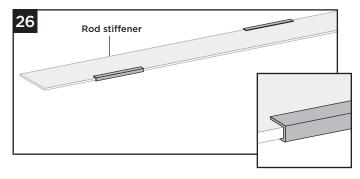
26. Attach tape (qty 6 provided) to alternating sides of the rod stiffener as shown.
