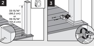
2. Measure up from decking surface 33-15/16" (86.2 cm) for 36" (92 cm) rail height or 39-15/16" (101.4 cm) for 42" (107 cm) rail height. Mark with light line.
