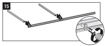
15. Attach **one** end vertical and **all** intermediate verticals to bottom rail using HZ spacer and screws provided. HZ spacer should be oriented so the ribbed side of the spacer is not showing.
