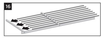
16. Slide all rods through intermediate supports and into end vertical support.
