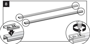
8. Place HZ template at end of top and bottom rails. Pre-drill pilot holes (using a 7/64" bit or small punch) at locations.
