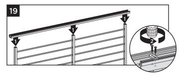
Install top rail to all vertical and end supports using HZ spacer and screws provided. HZ spacer should be oriented so the ribbed side of the spacer is not showing.
