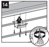
NOTE: Pre-drilling before attachment is recommended.
