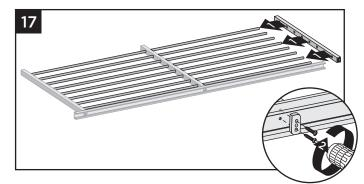
17. Slide end vertical onto rods and attach to bottom rail using HZ spacer and screws provided. HZ spacer should be oriented so the ribbed side of the spacer is not showing.
