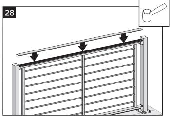
28. Using a mallet, install top rail cover.
