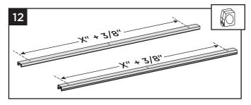
Measure the distance between the end (outer) holes (X") on top or bottom rail and add 3/8" to this measurement.
