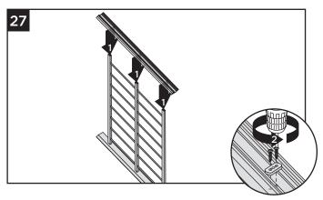
27.Install top rail to all vertical and end supports using S Wedge Spacer and screws provided.
