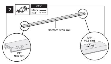
Cut each end of the bottom stair rail and bottom rail cover 1/4" (0.6 cm) shorter than the mark on each end to allow for fit into bottom stair rail brackets.
