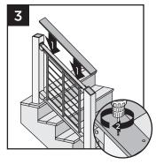
NOTCH CUT ON THE UNDERSIDE OR SLIGHT PLANING ON THE UNDERSIDE TO ALLOW DECK BOARD TO CLEAR TOPS OF BRACKETS AND SIT FLUSH ON TOP OF POSTS AND RAILS. Attach boards on each post with Trex-recommended composite screws (quantity of 2 per each post/board end).
