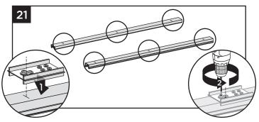
21. Using the slot on the HZ template, locate marked line and drill two 7/64" pilot holes at each mark (or mark with a punch).
