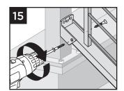
16. For stair crossover post configuration, fasten upper stair rail to swivel crossover post bracket by installing screws diagonally through crossover stair bracket into upper rail using two self-tapping screws (provided) on each side.
