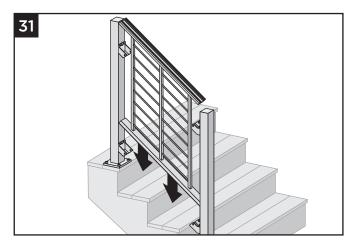
31.Drop assembled stair rod rail panel into brackets.
