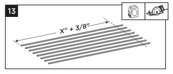
13. Cut rods to the length measured in previous step.
