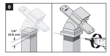
8. Once location/height is determined, center and predrill two holes (using a drill bit slightly smaller than that of self-tapping screw diameter) on opposite sides of post, approximately. 1/4" (0.6 cm) from top of post. Drill through the post and into the stair crossover swivel bracket on each side.
