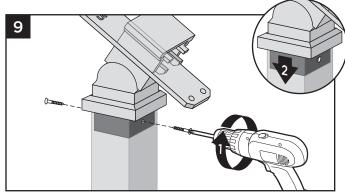
Attach stair crossover swivel bracket to post with two self-tapping screws (provided). Slide cover over post to hide screws.
