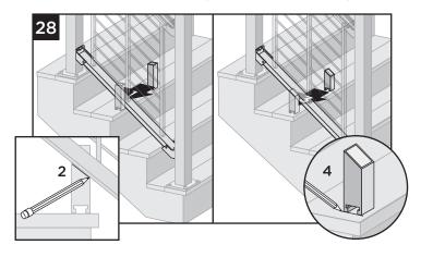
28.Temporarily drop assembled stair rod rail panel into brackets. To ensure proper location place foot block towards the nose of the stair tread along the side of the bottom rail. Mark location of angle on foot block and cut on mark. Then place foot block under the center of the bottom rail. Mark placement location of the base.
