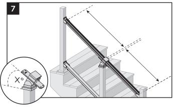
7. Determine location/height of the stair crossover swivel bracket by aligning the angle of this with the fixed brackets already installed. Note that the crossover post may need to be cut to ensure the top stair rail is parallel to the bottom stair rail.
