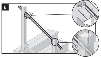
Position top rail to side of post. Mark top stair rail at each location stated. On UPPER STAIR POST, mark from underside of bottom rail. On LOWER STAIR POST, mark from topside of bottom rail.
