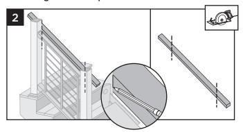
2. Place 2 x 4 beside top rail. Mark and cut (both ends need to be cut on an angle for proper fit).
