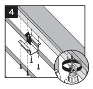
NOTE: Pre-drilling before attachment is recommended.
