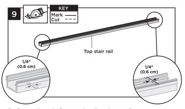
Cut each end of top stair rail and top rail cover 1/4" (0.6 cm) shorter than mark to allow for fit into top stair rail bracket.
