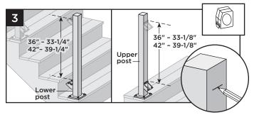
3. On Lower Post - From top of lower bracket, measure up and mark with light line (33-1/4" for 36" rail; 39-1/4" for 42" rail). On Upper Post - From top of lower (upper) bracket, measure up and mark with light line (33-1/8" for 36"rail; 39-1/8" for 42" rail).
