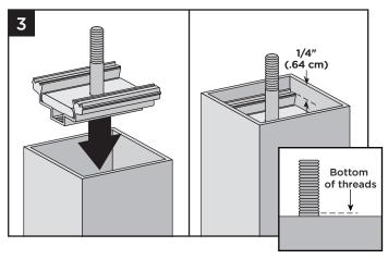
Insert assembly (from step 2) into the top of post.
