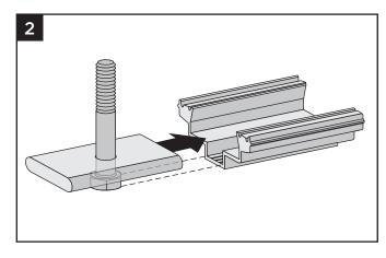
2. Align and insert the wedge plate with bolt into the v-wedge. Slide the wedge plate in until the ends are flush with the ends of the v-wedge.
