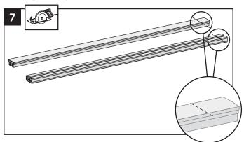
7. Cut both bottom and top rails to length as determined above.
