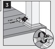
Measure up from decking surface 33-15/16" (86.2 cm) for 36" (92 cm) rail height or 39-15/16" (101.4 cm) for 42" (107 cm) rail height. Mark with light line.
