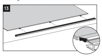
13. Lay glass on clean soft surface and install the bottom sill gasket onto the bottom edge of the glass panel.
