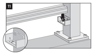
11. Place adhesive strips (provided) into bottom rail brackets, and then place bottom rail into brackets.
