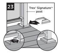
22.Attach corresponding bracket covers over opening in top and bottom rails.
