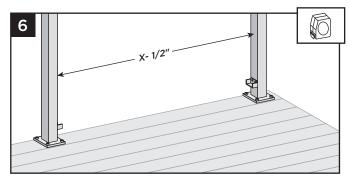
6. Measure distance between posts (X), and subtract 1/2" for bracket clearance.
