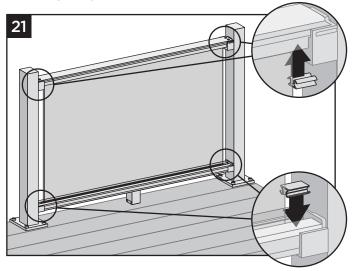
21.Cut snap-in channel filler to correct length and install into channels of bottom and top rails. Use of a rubber mallet may assist with this step. **DO NOT** attempt to cut short snap-in pieces with a miter saw. Use an angle grinder or hack saw only.
