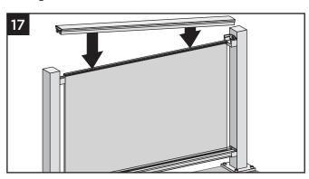
17. Starting at one end and working down, press the top rail firmly onto the top of the glass panel (with top head gasket on glass). Ensure the top rail is centered properly and top rail will seat into brackets when finished.
